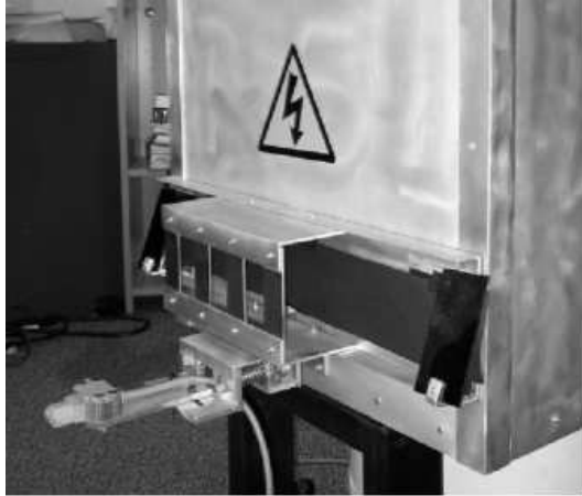
Figure 1: The ANU Recharging Station
